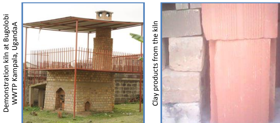
Figure 10: FS re-use options - FS Burning to fire clay bricks
