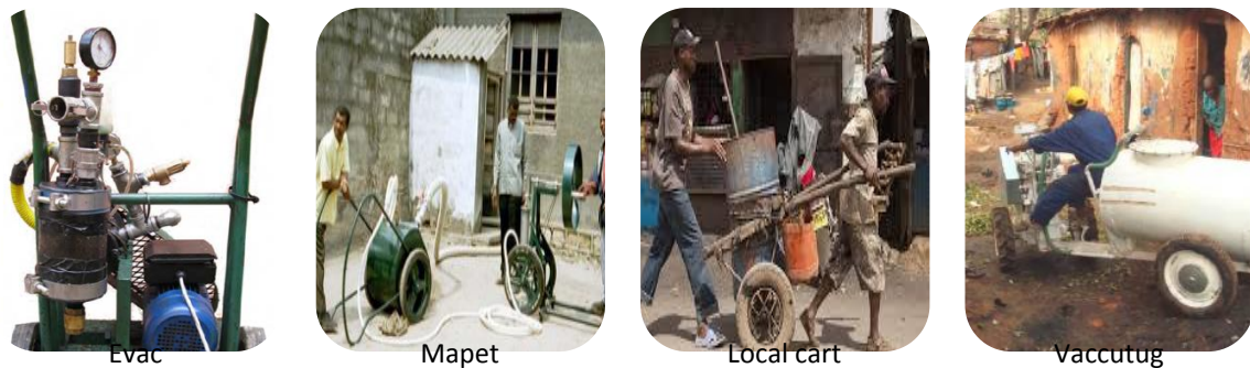
Figure 4: Semi-mechanized pit emptying
