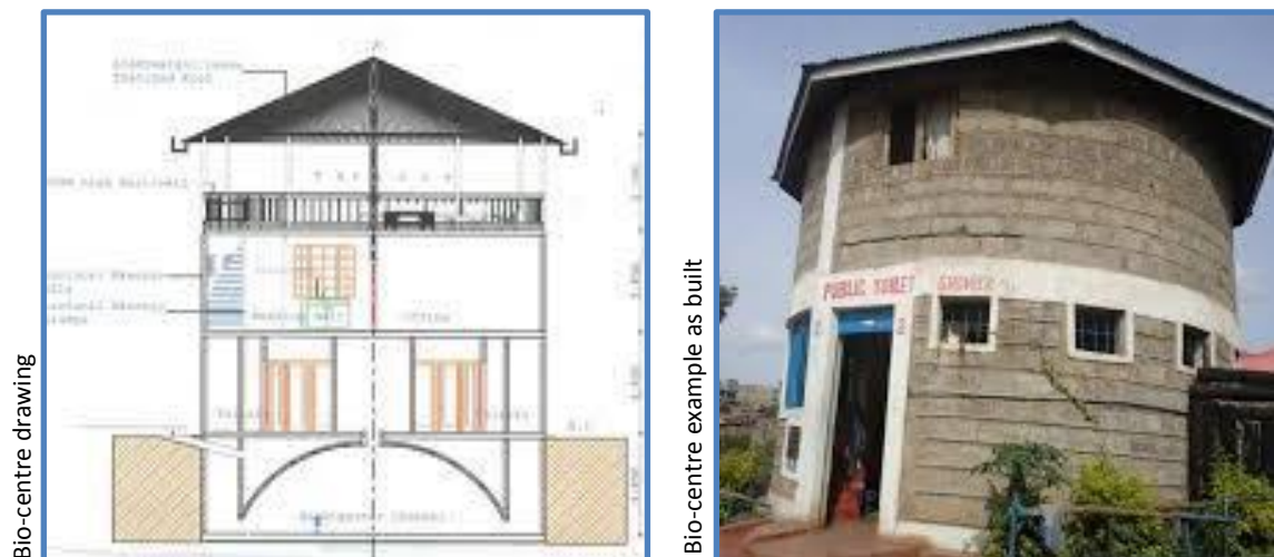
Figure 9: Typical Bio-centre in Kenya - drawing and As built
